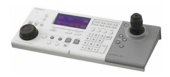
An optional RM-NS1000 System Controller - which connects to the NSR-1000 Series or a client PC via USB cable - allows the user to control multiple servers and cameras. A wide range of operations can be performed from this unit, including camera selection, Pan/ Tilt/Zoom (PTZ) with preset controls, snapshot capturing, video exporting, and event search and playback.
